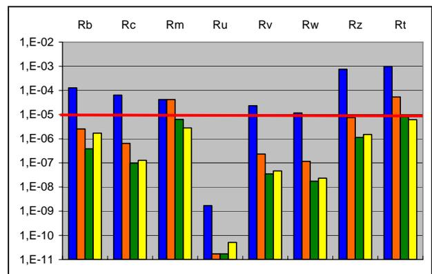
Figure 8 - Influence of LPS and storm detector on risk parameters in example N°2
