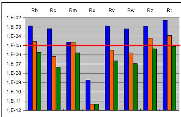
Figure 7 – Influence of LPS and storm detector on risk parameters in example N°1
