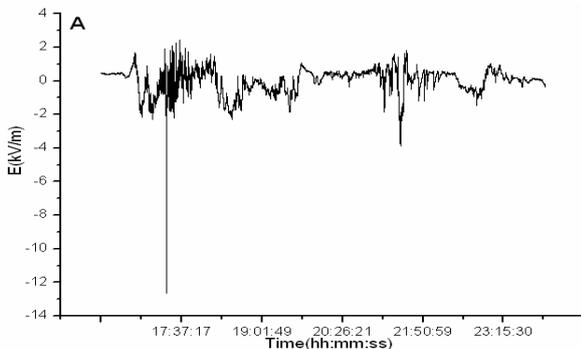
Figure 5 – Difference of measured electrical field during one thunderstorm on July 21, 2007
