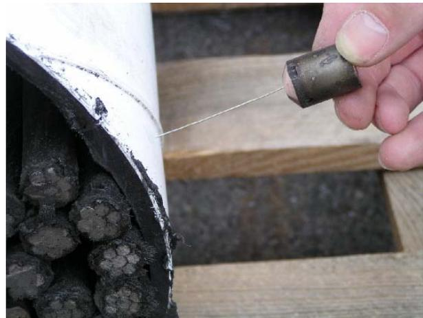
Fig. 2. Fuse wire connected to one of the strand inside the duct
