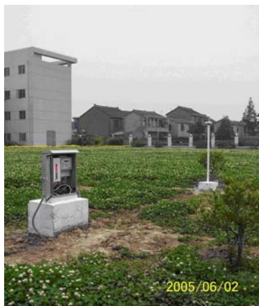
Fig. 5 – one of the local storm detectors in test in the open air laboratory
