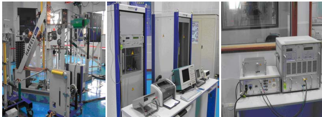
Fig. 1 – Example of testing means for SPDs in SHLPC (from left to right 200-180 impulse current generator, PSURGE 30.2 and PSURGE 6.1 Surge Generators)
