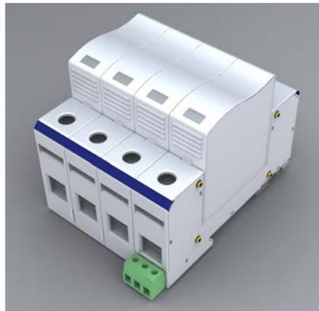
*Figure 1: Patented technology developed by Iskra Zascite and incorporated into its Safetec product line of AC and DC SPDs uses “arc-lengthening” in its disconnecter design, in conjunction with thermal current limiting components, to help control the follow-current while disconnecting on DC. The series meets IEC and UL standards.*
