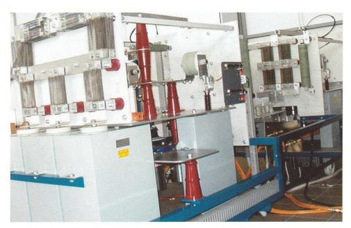
Our Lightning and Surge Current Generator is able to produce, apart from the typical wave shapes  $8/20~\mu s$ ,  $8/80~\mu s$  and  $10/350~\mu s$ , surge currents of any wave shape within front time  $T_t=4$  and tail time  $T_t=20~\mu to$  500 us.
