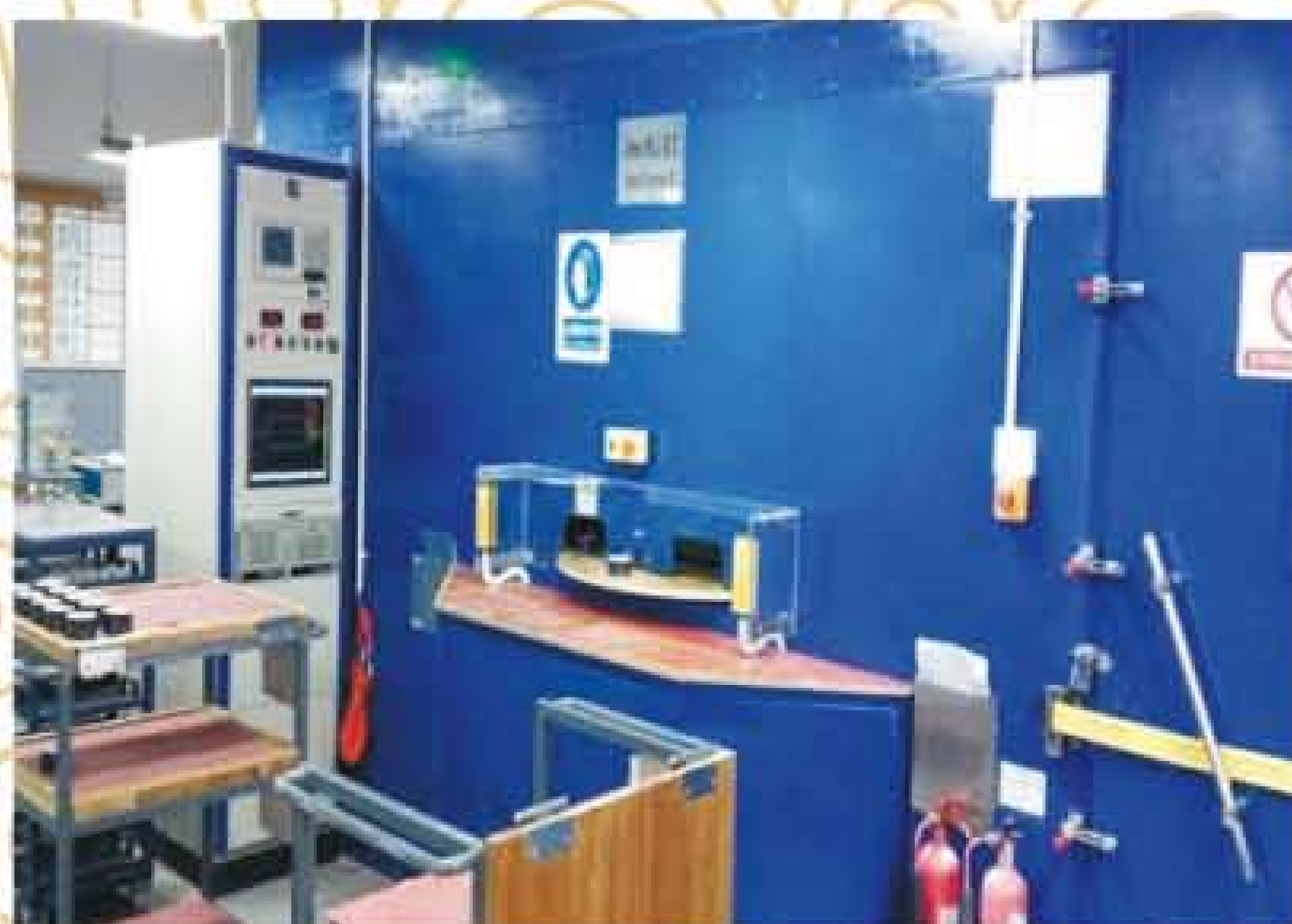
2ms 2kA Long Duration MOV Test System
