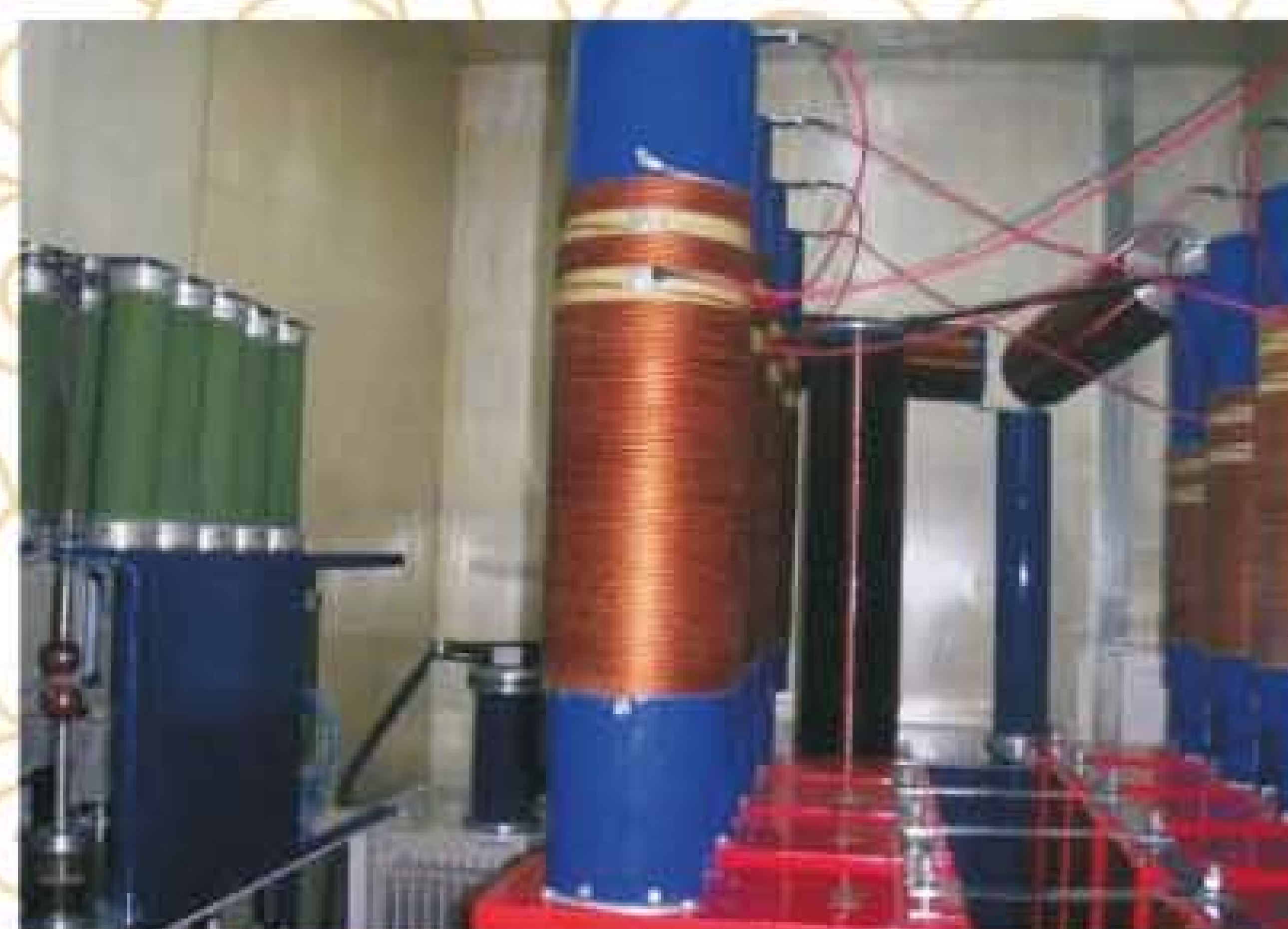
2ms 1kA Long Duration MOV Test System
