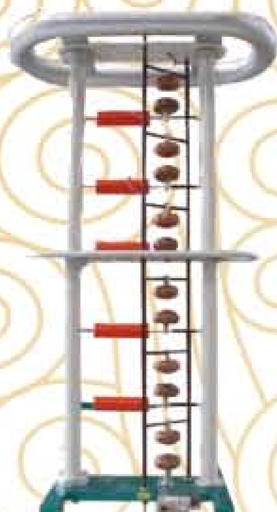
1200kV Chopping Gap for Transformer Testing
