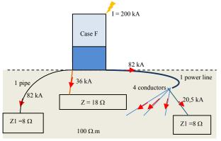
Figure 5 : Iimp current in SPD (connection type CT1, LPL I, using formula 2) - case F
