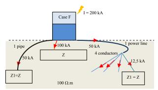
Figure 6 : Iimp current in SPD (connection type CT1, LPL I, using 50/50 rule) - case F
